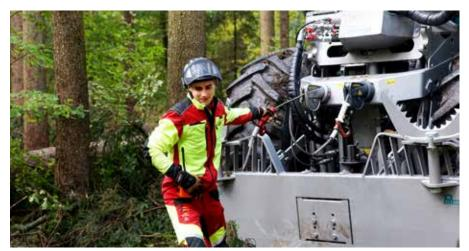
On the Pm Trac, Pfanzelt's winch units are mounted under the forest crane above the rear axle.
