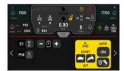
In addition to the preselection of speed and start-up characteristic, an automatic switch-on and switch-off can also be preset in the PTO management.
