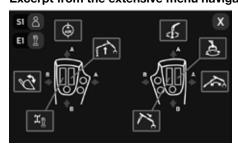
Adapted to the driver; he can individually preselect the assignment of all joystick functions and operating levers for hydraulic control units at the operator station, and save them in the driver management system.
