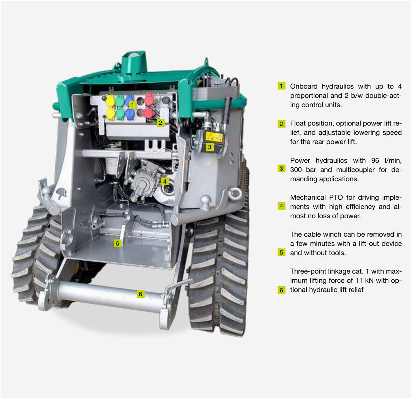
**1** Onboard hydraulics with up to 4 proportional and 2 b/w double-acting control units.
